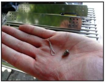
Save the cotter pin, as well as the bolt that the cotter pin mounts through. Set them aside in a safe place as you will be reinstalling those parts on the new burner.
