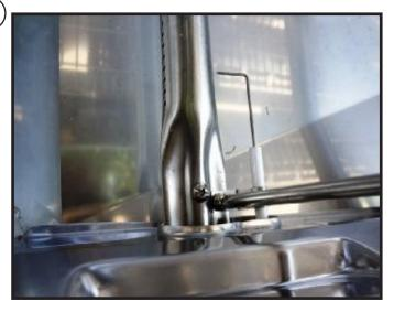
Secure the ignition mounting bracket back to the burner mount. Make sure the ignition wire is 1/8th of an inch away from the main burner, and aimed at the top of a hole in the burner.
