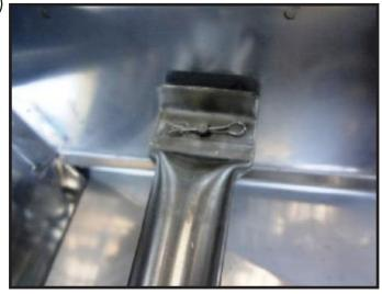
Place the cotter pin through the bolt's end protruding through the top of the burner. You may now release your hold on the bolt as it is held in place by the cotter pin. Bend the end of the cotter pin as to lock the burner in place.
