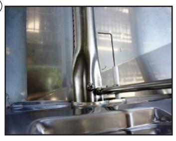
Remove the screw that mounts the ignition electrode to the main burner. The bracket and electrode should be shifted aside slightly as to not be damaged when removing and replacing burner.
