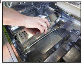
Repeat steps 4 - 15 for each additional burner that needs to be replaced. When you are finished replacing all of the burners, replace the flame tamers over the burners. Set each flame tamer evenly over each of the burners.
