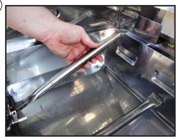
Place the front end of the burner into the recess at the front of the bowl assembly first.
