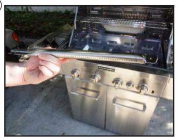
Locate the new burner that you wish to install into the grill.
