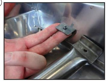
Slide the cotter pin bolt into the bottom of the bracket where the burner mounts. Hold the bolt in place from below.
