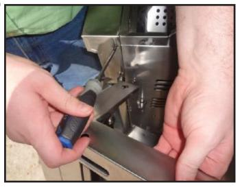
Remove the screws from the side of the control panel where the gas flex line extends towards the shelf with a side burner. Be careful not to kink or otherwise damage the flex line.
