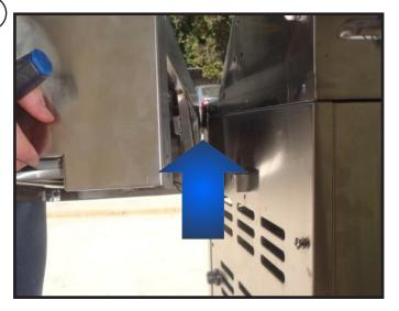
Remove the side shelf with a burner, using the keyhole slots on the left and right posts just as you did in Step 6. The burner has a flex gas line attached, so extra care must be taken to avoid damaging the flex line.
