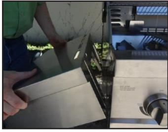
Remove the side shelf without a burner, using the keyhole slots on the left and right posts where you loosened the screws on Step 2 to slide over the head of the loosened screws.
