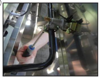
Install the replacement valve onto the manifold, placing the valve stem through the hole in the control panel. Hook the manifold retainer bracket to the manifold and tighten the screw to secure the bracket. Repeat steps 16 – 21 for each valve that needs to be replaced.
