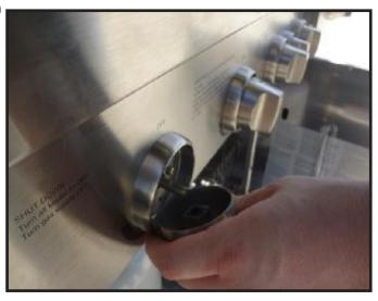
Remove the control knobs from the grill. You may need to remove a screw to complete this process and will need a 5/64 Allen key to complete this step. Repeat this step for each of the knobs on the main control panel where valves need to be replaced.
