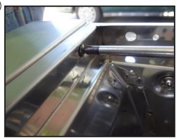
Re-install the screws on the inside lip of the main bowl area where the cooking grids set into. These screws will help support and secure the control panel. those components.
