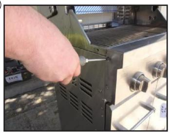
Remove the screws from the side of the control panel where you removed the shelf without a burner.
