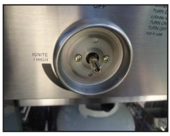
Mount the bezel and the screws to the valve on the front of the control panel centered around the valves stem. Repeat this step with all valves that had been replaced.
