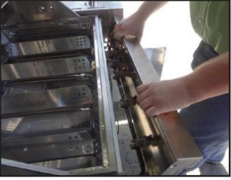
Free the control panel from the main body of the grill. There are still going to be component parts of the grill that are connected to the control panel, so take extra care with this step to avoid damaging those components.
