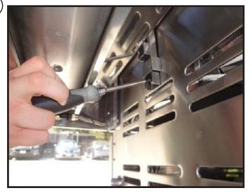
Secure the screw that goes into the center post of the side shelf, and then tighten the screws that mount on the left and right via the keyhole slots. Repeat steps 30 and 31 for the un-mounted side shelf on the opposite side.
