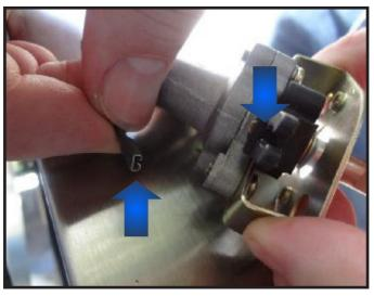
If you have recently applied a soapy water solution to the valve, clean the solution from the valve before completing this step. Remove the junction wire from the valve connection, mounted above the main body of the valve.
