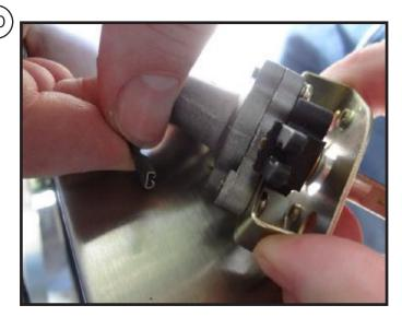
Replace the junction wire connection from the previous valve onto the replacement valve. The wire mounts above the main body of the valve.
