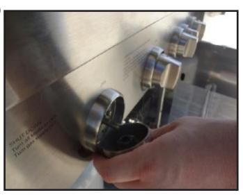
Reconnect the burner knob to the valve stem. Secure the screw if necessary by using an Allen key. Repeat this step for all valves that have been replaced. (28)
