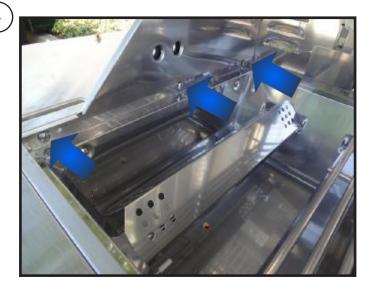
Locate the three screws that attach to the shelf from the inside of the main bowl assembly.
