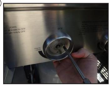
Remove the two screws from the bezel on the left and right side of the valve stem protruding from the center. Repeat this step for each of the bezels on the main control panel where valves need to be replaced.
