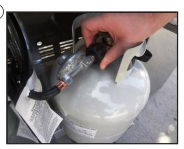
Remove the regulator coupling nut from the propane tank by turning the coupling nut counter-clockwise.
