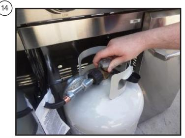
To pressurize the line, open the propane tank gas valve by turning it counterclockwise until it will no longer turn.
