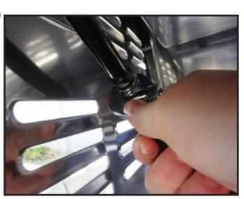
Using the two wrenches, tighten the brass fitting onto the manifold. Do not over-tighten the connection.
