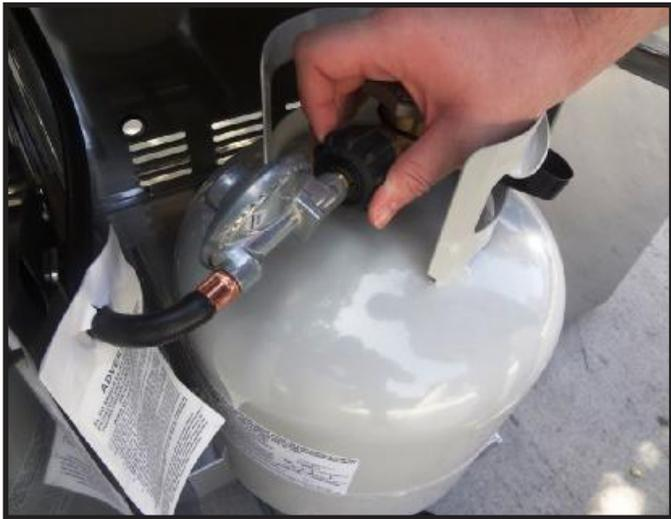
Re-attach the regulator coupling nut to the propane tank by turning it clockwise. Slowly open the propane tank gas valve and continue to turn the valve very slowly counter-clockwise until it will no longer turn.
