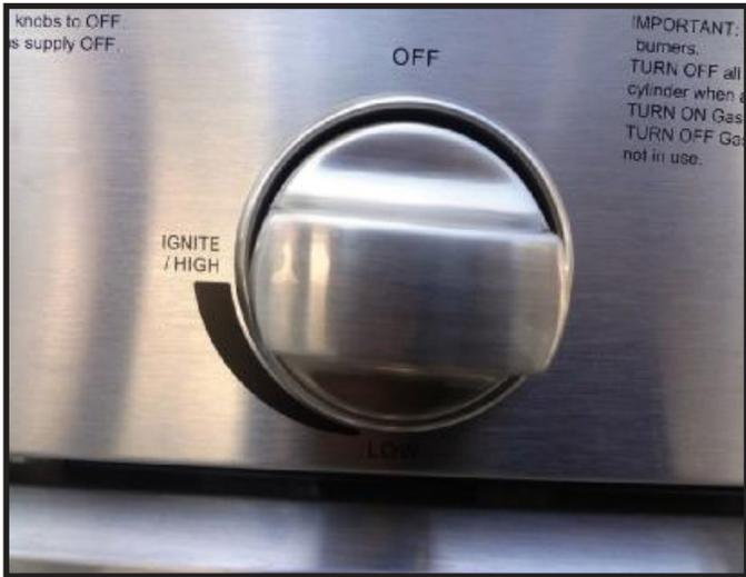
Turn all of the burner knobs to the 'IGNITE/ HIGH' setting for 10-15 minutes in order to bleed any gas from the gas line.
