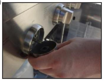
Gently pull the control knob to remove it from the valve stem.
