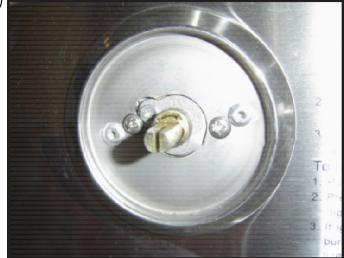
Once the knob has been removed, the valve stem will be exposed.
