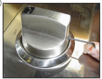
Use a 5/64ths allen wrench to release the screw that holds the knob.
