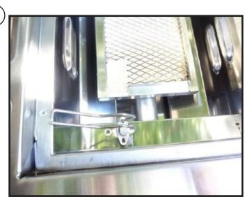
Now that the ignition electrodes are free, turn the part to the side so it will not interfere with the removal of your sear burner.
