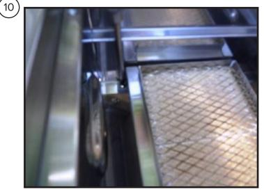
Reinstall the screws you removed in Step 5. Turn each of the screws a few turns into the threading, but do not tighten until all screws have been affixed to the unit.
