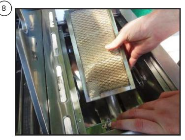
Place the searing side burner into the bowl where it mounts. The burner tube at the bottom-front of the unit should be aimed to go into the hole in the front of the bowl assembly.
