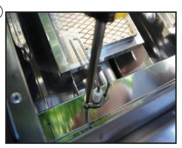
Install the screw to the ignition electrode removed on step 2. Make sure that the ignition is placed over the searing side burner near the opening in the grate of the burner.
