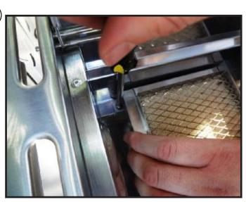
Remove the screws that mount the sear burner to the back of the grill. Save these screws as they will be required to install the new unit.
