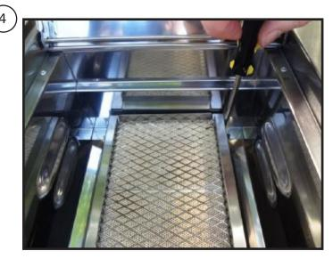
At the back of the bowl assembly where the sear burner is seated, locate the two screws where the unit mounts. Some units also have a screw that secures the unit closer to the front.
