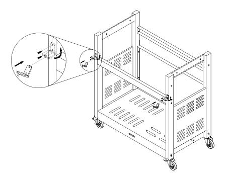
**Step 6:** Assembly the door in the fix piece of door shaft from bottom as shown figure and tighten the screws.
