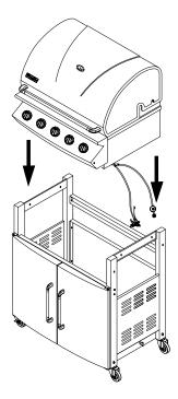
**Step9**: Open the lid ,take out the cooking grid first, then screw tighten the four(4) pcs 1/4\*12 screws into the left side and right side of firebox as shown figure below.
