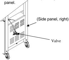
Step 3: Insert valve stem assembly into burner venturi.
