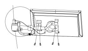
Step 2: Remove 4(four)screws & washer from the "U" . brackets on the side burner.
