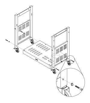
**Step 3**: Assemble the back panel to the two side panels. with two (2)pcs 1/4\*12mm screws and four (4) pcs 5/32\*12 as shown figure below.
