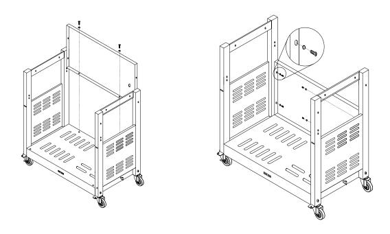
Step 4: Assemble the front cart flame and back cart flame to the front side and back side of the side panel with eight (8) screws. Attention: The front cart flame should be screwed from outside into inside with four(4) pcs 1/4\*42 screws, and the back cart flame should be screwed from inside into outside with four(4) pcs 1/4\*12 screws.
