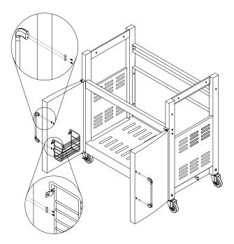
Step8: Remove the head unit of grill from carton. Insert the upper portion of the grill onto the cart from the top. Caution!! The firebox is heavy, and we recommend two or more people to lift up firebox.
