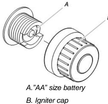
2. Remove battery from the battery compartment.
