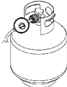
5. Using your hand, turn the gas pressure regulator/hose assembly clockwise to connect to the 20 lb LP gas fuel tank as shown.
