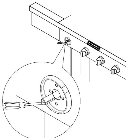
3. Check that burner operates at the new high flame setting. It may be necessary to adjust the screw setting slightly more to get the ideal burner flame height.
