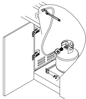
6. Use an adjustable wrench to install the Natural gas regulator hose to the manifold and secure. Attach the Natural gas regulator to the side panel inside the grill cart with the two screws that are preassembled on the regulator.
