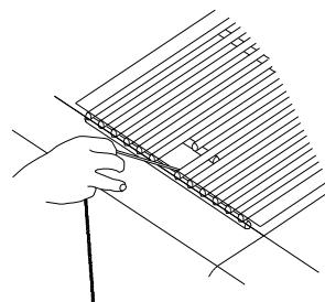
6. Push in and turn the burner knob to IGNITE/HIGH for the burner closest to the lit match. The burner will light immediately. When burner is lit, turn knob to desired setting.
