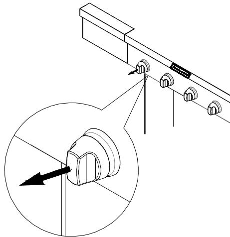
2. Use a flat-blade screwdriver to turn the high flame setscrew counterclockwise approximate 90°.
