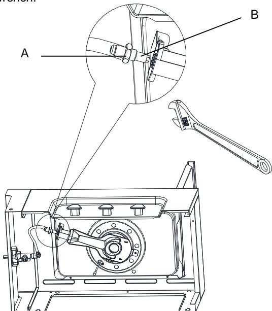
A. Side burner orifice brass connector
