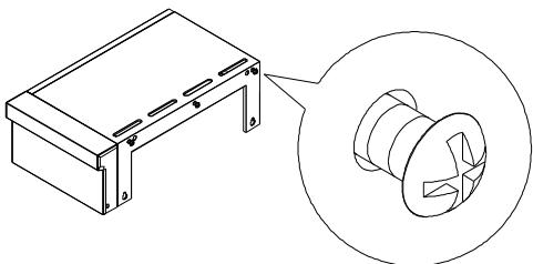
4. Loosen 2 screws on the grill side panel but not remove them completely and remove 1 screw on the grill control panel.
