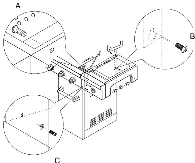
8. Remove the 2 screws from side burner valve assembly. See illustration step 10.
