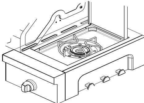
6. Push in and turn the control knob to IGNITE/HIGH. For the burner closest to the lit match. The burner will light immediately. When burner is lit, turn knob to desired setting.
