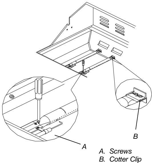
3. Use a flashlight to inspect into the burner through the burner inlet to ensure there is no blockage. If any obstruction is seen, use a metal coat hanger that has been straightened to clear them.
