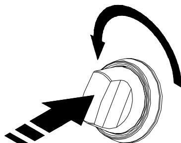
4. You will hear the "snapping" sound of the spark. When burner is lit, release the knob. Turn knob to desired setting.
