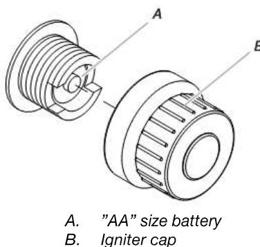
3. Remove battery from the battery compartment.
