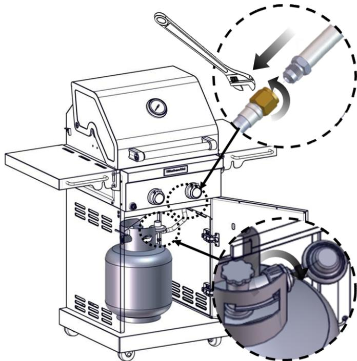
6. Use an adjustable wrench to install the Natural gas regulator hose to the manifold and secure. Attach the Natural gas regulator to the side panel inside the grill cart with the two screws that are preassembled on the regulator.
