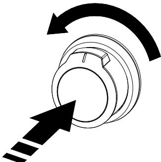
4. You will hear the "snapping" sound of the spark. When burner is lit, release the knob. Turn knob to desired setting.
