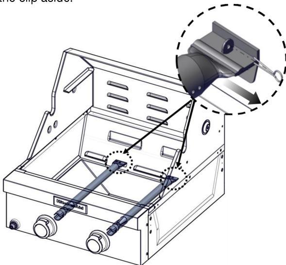
3. Remove the burner from the grill by lifting the burner out.
