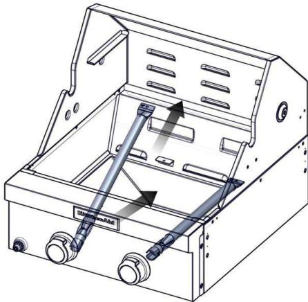
3. Use a flashlight to inspect into the burner through the burner inlet to ensure there is no blockage. If any obstruction is seen, use a metal coat hanger that has been straightened to clear them.
