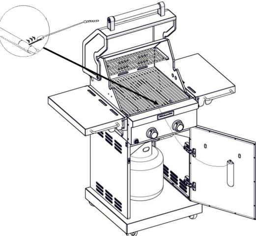
6. Push in and turn the burner knob to "🔥" for the burner closest to the lit match. The burner will light immediately. When burner is lit, turn knob to desired setting.
