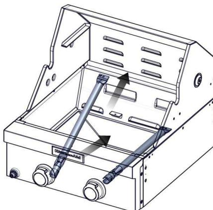
7. If flame is yellow (not enough air), turn air shutter adjustment screw counterclockwise.
