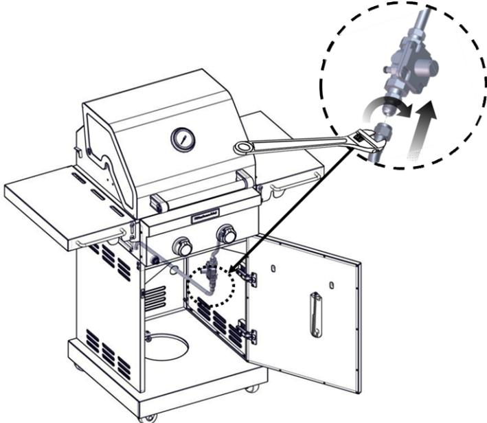
3. Connect the quick connector on the other end of the 10 ft (3.0 m) PVC flexible gas supply hose to the rigid Natural gas supply pipe.
