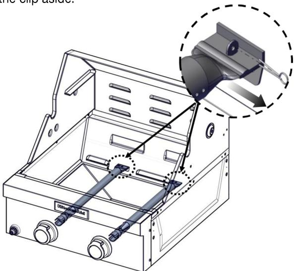
6. Remove the burner from the grill by lifting the burner out
