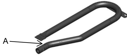
A. Air shutter adjustment screw
