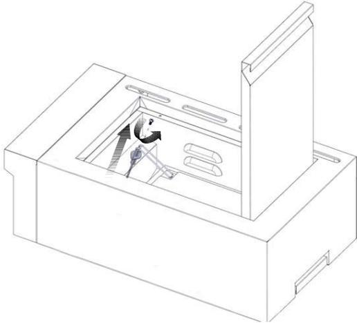
2. Remove two screws on the rear of the searing burner. Lift the burner starting from the back, as shown.
