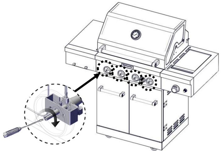
3. Check that burner operates at the new high flame setting. It may be necessary to adjust the screw setting slightly more to get the ideal burner flame height.
