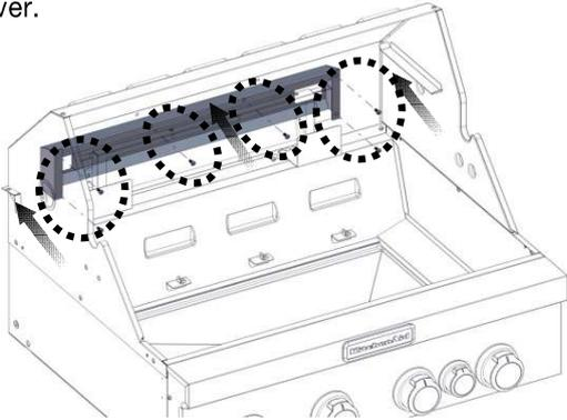
12. Reinstall the rotisserie burner heat shield and tighten the two screws.
