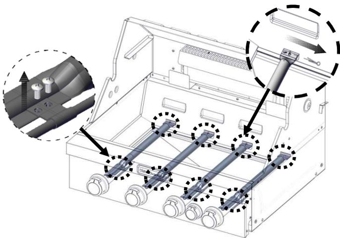
6. Remove the burner from the grill by lifting the burner out
