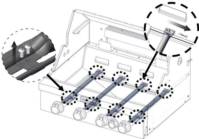
**IMPORTANT:** Check that the LP orifice is properly removed inside of the burner opening.
