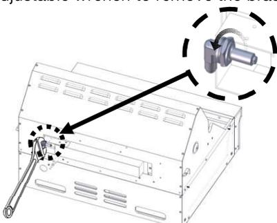
6. Use a 6 mm socket wrench or 6 mm nut driver to remove the orifice.
