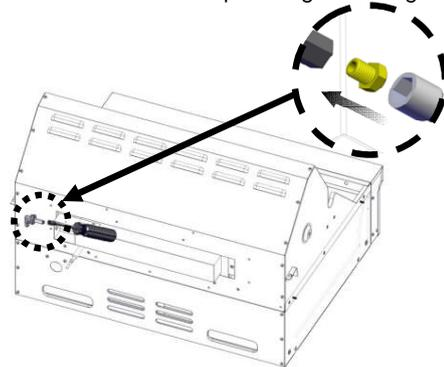
**IMPORTANT:** Check that the NG orifice is properly installed inside the valve.
