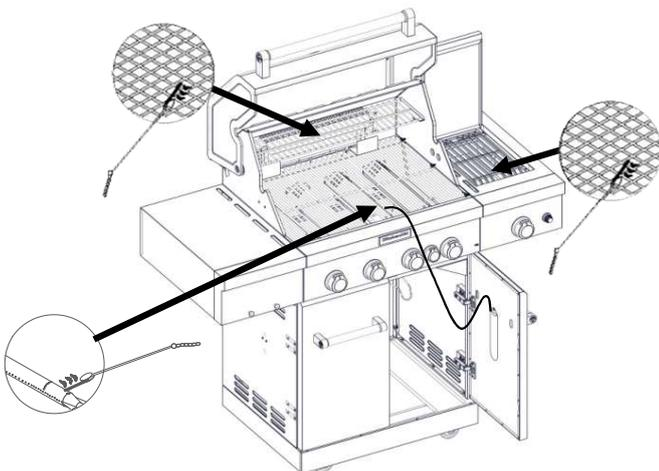
6. Push in and turn the control knob to "●". For the burner closest to the lit match. The burner will light immediately. When burner is lit, turn knob to desired setting.
