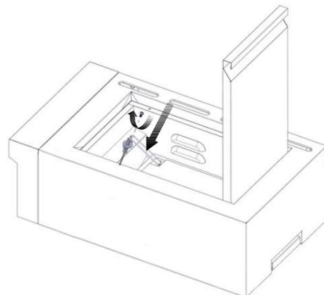
8. Open the manual shutoff valve in the gas supply. The valve is open when the handle is parallel to the gas pipe.
