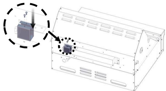
10. Reinstall the rotisserie burner rear cover.
