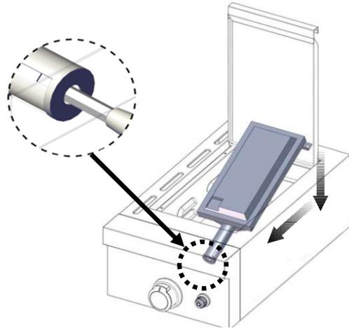
6. Reinstall the two screws to the rear of the searing burner.
