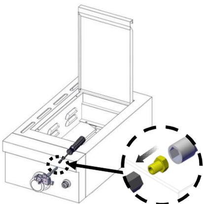
**IMPORTANT:** Check that the NG orifice is properly installed inside of the valve.
