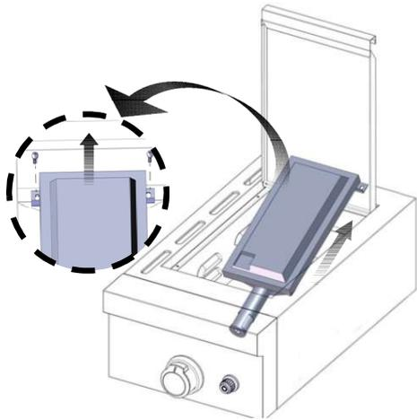
3. Use a 6 mm socket wrench or 6 mm nut driver to remove the orifice.
