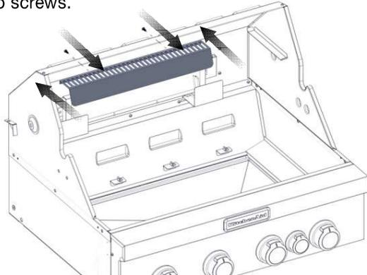
2. Use a flat-blade screwdriver to turn the high flame setscrew counterclockwise approximately 90°.
