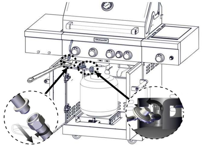
6. Use an adjustable wrench to install the Natural gas regulator hose to the manifold and secure. Attach the Natural gas regulator to the side panel inside the grill cart with the two screws that are preassembled on the regulator.
