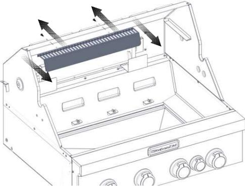
2. Remove the six screws on the rotisserie burner rear cover.
