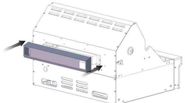
11. Reinstall the four screws onto the rotisserie burner rear cover.
