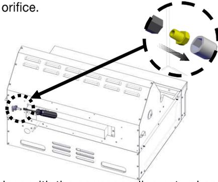
7. Replace with the corresponding natural gas orifice.
