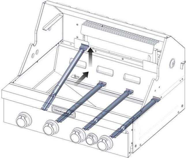
3. Use a flashlight to inspect into the burner through the burner inlet to ensure there is no blockage. If any obstruction is seen, use a metal coat hanger that has been straightened to clear them.
