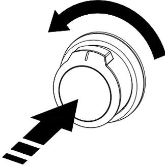
**IMPORTANT:** If burner does not light immediately, turn the burner knob to "O" and wait 5 minutes before relighting.
