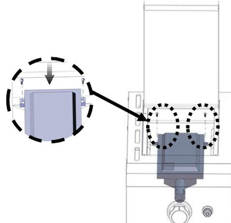
7. Use a screwdriver to reinstall the igniter pin.
