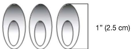
Check that burners are not blocked by dirt, debris, insect nests, etc., and clean as necessary. If they are clean, adjust air shutters as needed.
