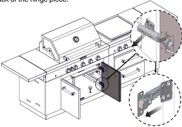
After detaching the bottom hinge, repeat for the top hinge. It will be necessary to support the door during this process.
