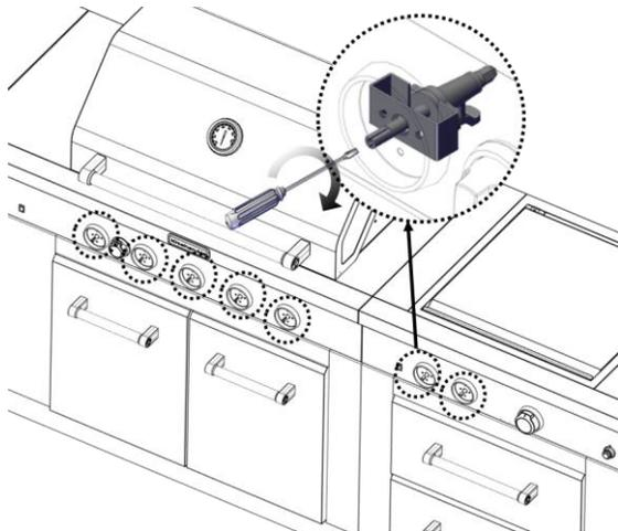
3. Check that burner operates at the new high flame setting. It may be necessary to adjust the screw setting slightly more to get the ideal burner flame height.
