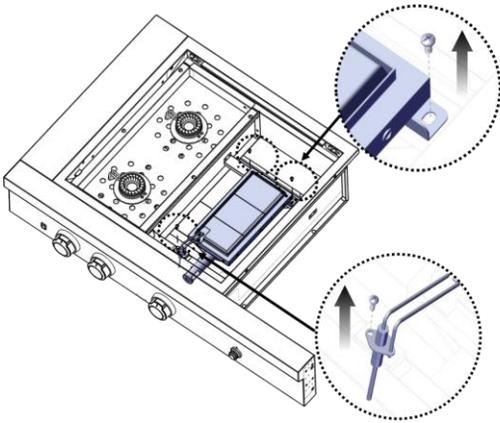
4. Lift the burner starting from the back, as shown.
