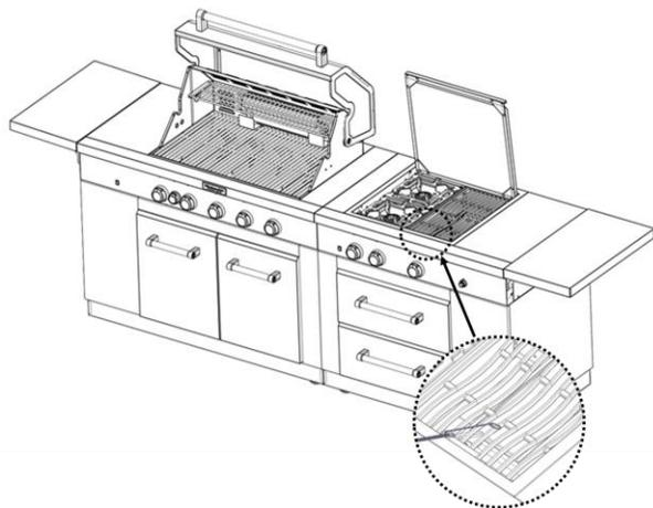
6. Push in and turn the control knob to "●". For the burner closest to the lit match. The burner will light immediately. When burner is lit, turn knob to desired setting.
