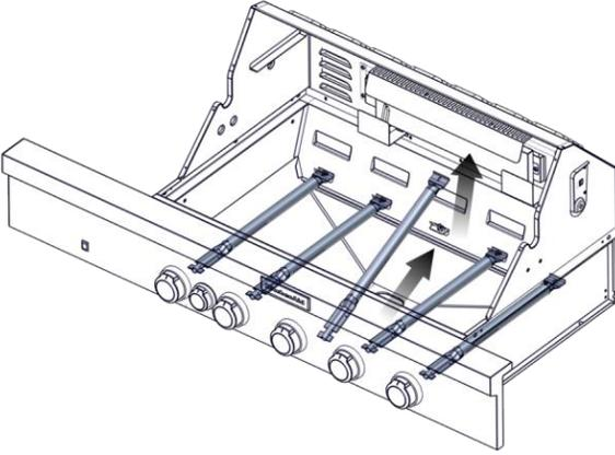
3. Use a flashlight to inspect into the burner through the burner inlet to ensure there is no blockage. If any obstruction is seen, use a metal coat hanger that has been straightened to clear them.
