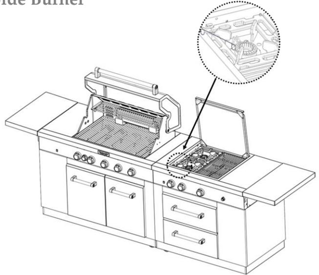
6. Push in and turn the control knob to "🔥". For the burner closest to the lit match. The burner will light immediately. When burner is lit, turn knob to desired setting.
