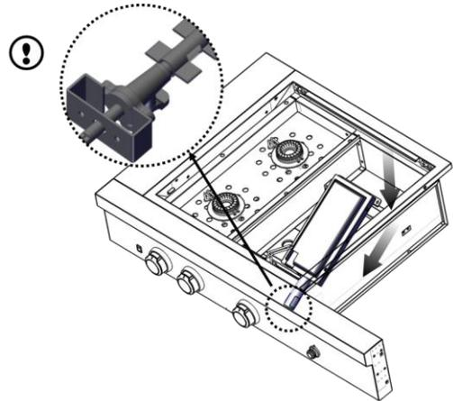
7. Reinstall the two screws to the rear of the searing burner. Reinstall the igniter pin.
