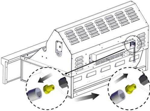
**IMPORTANT:** Check that the NG orifice is properly installed inside the valve.
