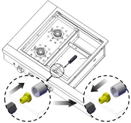
**IMPORTANT:** Check that the NG orifice is properly installed inside of the valve.
