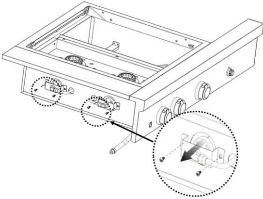
2. Use a 6 mm socket wrench or 6 mm nut driver to remove the orifice and replace with the natural gas orifice.
