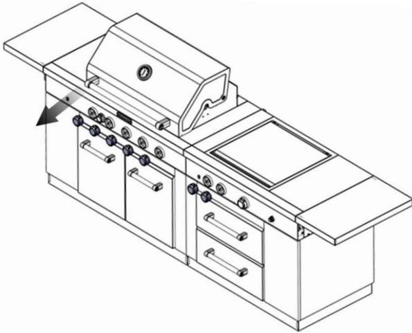
2. Use a flat-blade screwdriver to turn the high flame setscrew counterclockwise approximate 90°.
