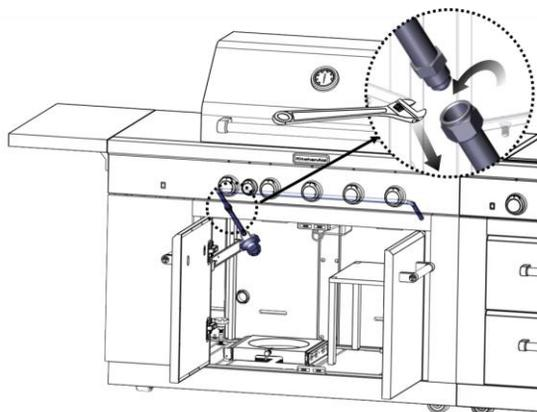
6. Use an adjustable wrench to install the Natural gas regulator hose to the manifold and secure. Attach the Natural gas regulator to the side panel inside the grill cart with the two screws that are preassembled on the regulator.
