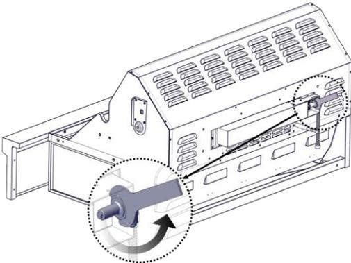
8. Reinstall the igniter bracket and tighten the screws.
