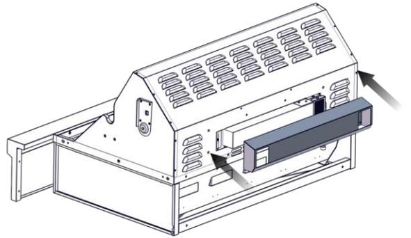
10. Reinstall the six screws onto the rotisserie burner rear cover.
