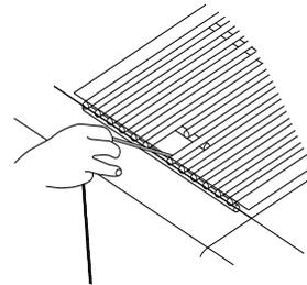
6. Push in and turn the burner knob to "🔥" for the burner closest to the lit match. The burner will light immediately. When burner is lit, turn knob to desired setting.
