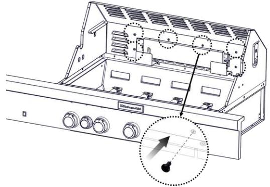
11. Reinstall the rotisserie burner heat shield.
