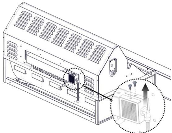
5. Use an adjustable wrench to remove the brass elbow.
