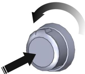
4. You will hear the "snapping" sound of the spark. When burner is lit, release the knob. Turn knob to desired setting.
