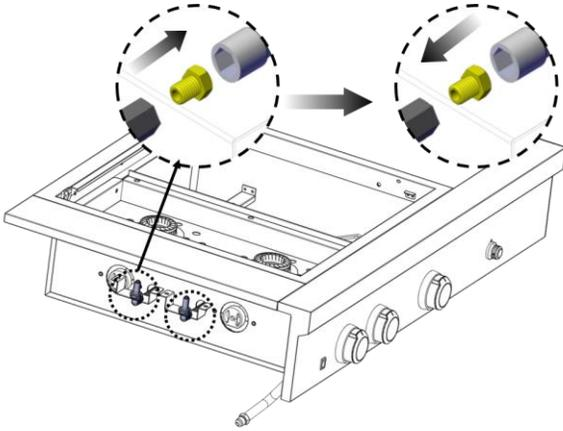
**IMPORTANT:** Check that the NG orifice is properly installed inside of the valve.
