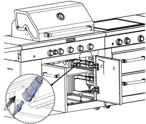
6. Open the manual shutoff valve in the gas supply. The valve is open when the handle is parallel to the gas pipe.
