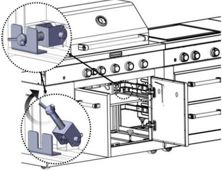
3. Use a screwdriver to remove screw from the igniter pin and two screws on the rear of the searing burner.
