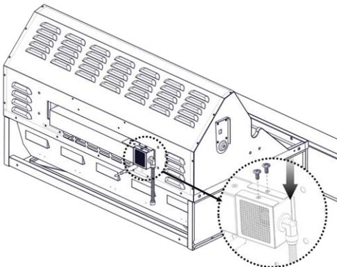
9. Reinstall the rotisserie burner rear cover.
